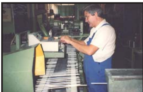
#5 Electrodes being checked for eccentricity.
