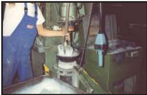
#2 Mixing the flux coating minerals for the electrode extruder.
