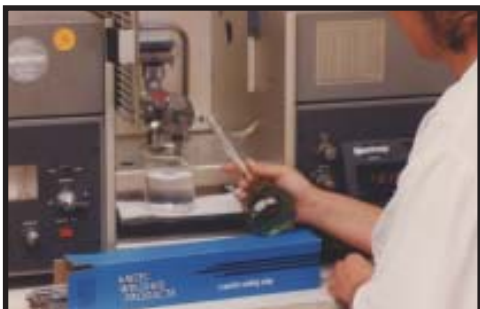
#10. The finished welding electrodes being tested by a photo-micrograph and photo-spectrograph for quality.
