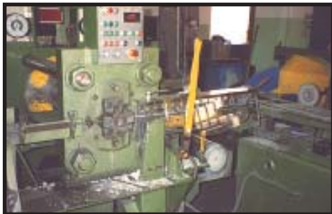
#3 Welding electrodes being extruded
