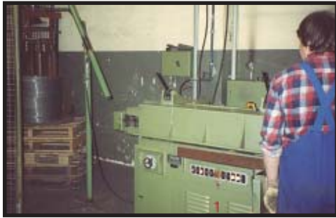
#1. Straightening and Cutting the Core Wire
